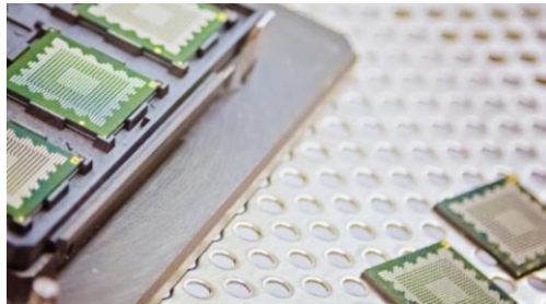
NAND Flash memory modules that use multiple memory dies arranged in a stack (up to 4 MLC / 3D MLC / 3D TLC dice)
